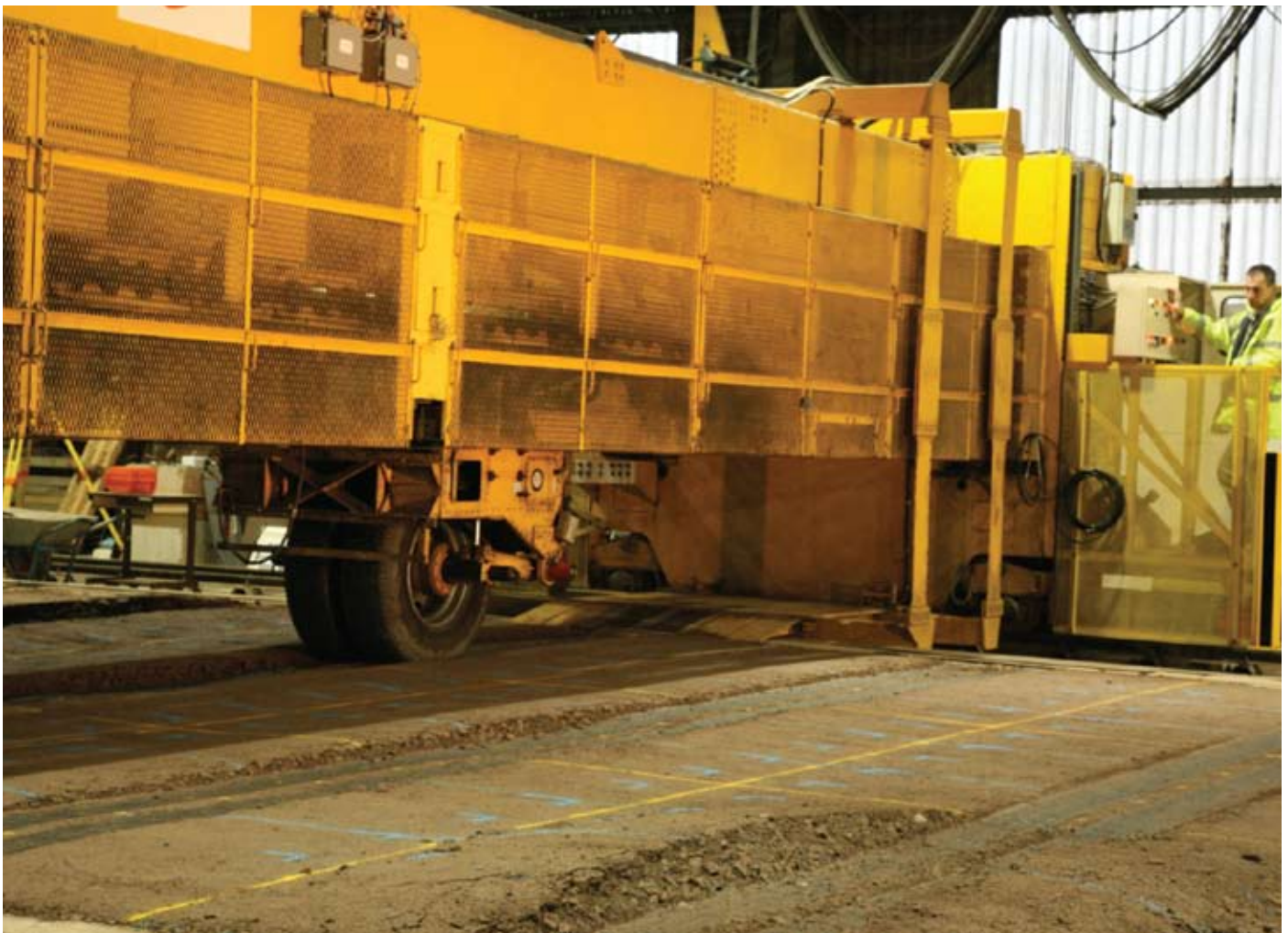
Extended trafficking testing performance trials at the Transport Research Laboratory are an essential part of demonstrating the in-ground performance of geogrids such as Tensar TriAx™.
