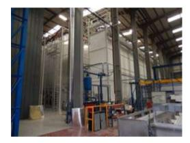
The new vertical paint line uses cutting-edge waste capture, energy efficiency and production planning technology and also features an integral vertical pre-treatment plant using the same 100% chromate free process that Smart uses with its existing horizontal paint line.
