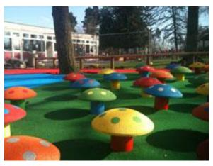
All Play Services worked with Leicestershire County Council to complete the project, where the Matchwinner Velour carpet by Playrite was installed directly onto a pre-prepared compacted base. Holes were created into the base for the toadstools to be fitted into and the carpet was cut to allow for them to fit in seamlessly. Matchwinner Velour comes in 12 bright colours, and the school chose green as shown in the image, as well as covering other areas of the playground in red and blue.
