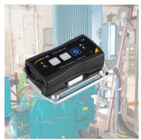
The PCE-VDL 16I has five integrated sensors for temperature, humidity, air pressure and light, as well as a 3-axis acceleration with a sampling rate of 1600 Hz.
