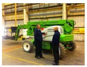
"At just 4,750kg for the HR17 and well under 6,500kg for the HR21, these machines are substantially lighter than other manufacturers' 45, 50 and 70 foot booms, meaning I can save on transport while offering customers lower point loadings too."
