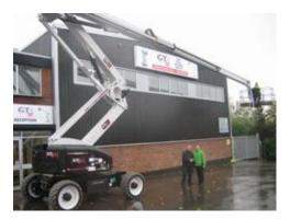
Niftylift's Tim Ward commented: "For the first time a 90 foot plus machine will not need a 'Low Loader' to move it to site. With the right specification, a 26 tonne truck can be used, offering the potential for huge cost savings for our customers."
