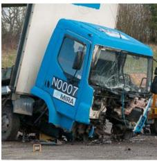
Heald recently tested the Mantis at MIRA's testing grounds, where it received a rating of PAS68:2013 Fixed Bollard V/7500(N2)/64/90:0.0/0.0. This means that the Mantis will arrest a 7.5 tonne truck from a speed of 64kph with zero penetration and zero dispersion. In the impact, the structure of the bollard remained intact, ensuring continued protection against further attack.
