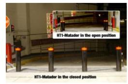
It is also important to note that because the moving bollard(s) slides to one side (rather than retracting into the ground); it is completely visible throughout its movement. Drivers will therefore be much more aware of the moving bollard's position and will not attempt to sneak through if they see
