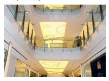
For this large-scale project, the architect called upon the company TTI Elektrik Elektronik, an approved Clipso fitter with excellent skills and innovative technical knowledge. A total of 1,100 m<sup>2</sup> of translucent coverings (ref. PT 507) and 1,000 m of profiles (ref. P-CC) were used to make the luminous ceilings. Four fitters were required for this project which took one month to complete.
