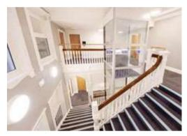
This model is designed to fit seamlessly into both new and existing buildings and in the Newcastle case, it was installed in the stairwell, to keep as much of the space as possible and help to maintain the building's original features. The glass shaft and panoramic doors of the lift preserve the natural light of the building.
