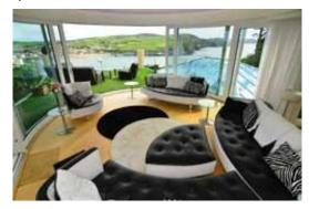
Forming a semi-circle that measures 8.4m in girth and maximising the 180-degree views, the curved door has 28mm Low-E toughened double glazed units. It opens onto a square terrace with a frameless structural glazed balustrade, also supplied by Balcony Systems. This balustrading style was chosen specifically to fulfil safety requirements with low-maintenance minimum visual impact, plus the added benefit of protection from prevailing winds.
