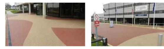
The client was looking for a hard wearing, low maintenance surface that would rejuvenate the existing 300 sq m concrete paved pedestrian area and selected a porous resin bound system in a bold design using two different colours.
